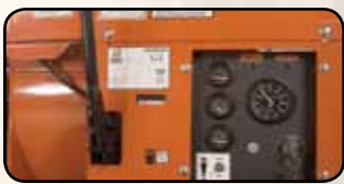
Belt engage lever is placed near control panel for easy monitoring of performance
