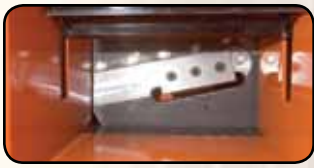
The large feed roller can be raised and lowered with a hydraulic jack
