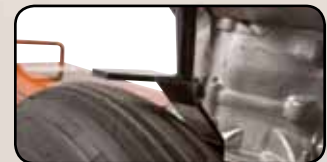
A single wheel brake allows the cutting head to pivot across the surface of a stump
